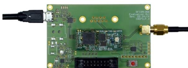
Picture 1 – Evaluation board equipped with RFID module
